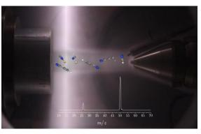
directly in the supersonic flow with the help of an electron gun [8-9].
